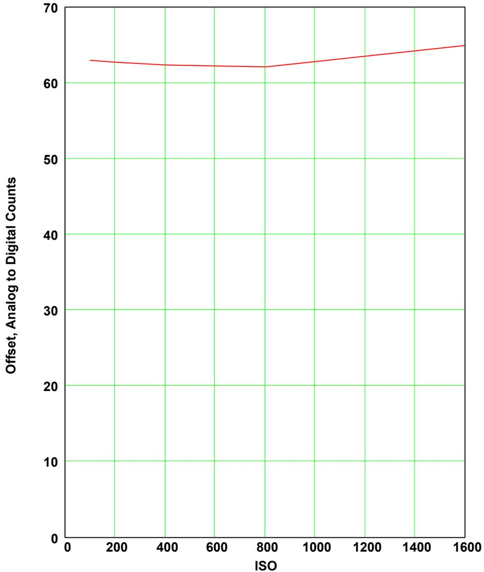
**Figure 3. The RAW image offset value in ADU present in EVOLT photos as a function of ISO setting. The image offset is essentially independent of ISO setting and is visible in detailed histogram displays of EVOLT images.**
