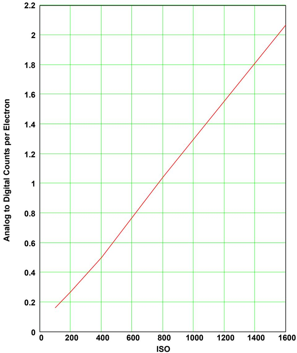
**Figure 1. The transfer characteristic of the Olympus E-300 EVOLT DSLR measured in analog to digital counts per photoelectron (ADU/electron versus ISO or gain setting). Note ~1 ADU/photoelectron at ISO = 800.**
