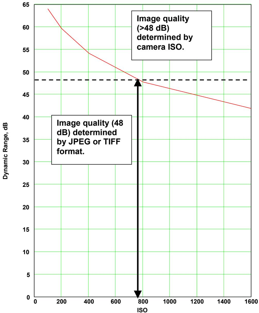
Figure 2. The maximum linear dynamic range of the Olympus E-300 EVOLT DSLR as determined by maximum linear exposure (CCD well storage and readout noise) and camera ISO setting (gain setting). The maximum linear dynamic range was measured to be 63.55 dB versus the CCD specification of 64.04 dB. **Note that both JPEG and TIFF image dynamic range are 48 dB (8 bits/color) and that around and above ISO 800, noise is visible in JPEG images.**
